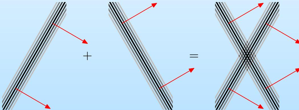
$$\left. \begin{array}{l} X \text{ pulses} \\ \text{Bessel pulses} \end{array} \right\} v_f = v_g = c/\cos\theta > c$$
